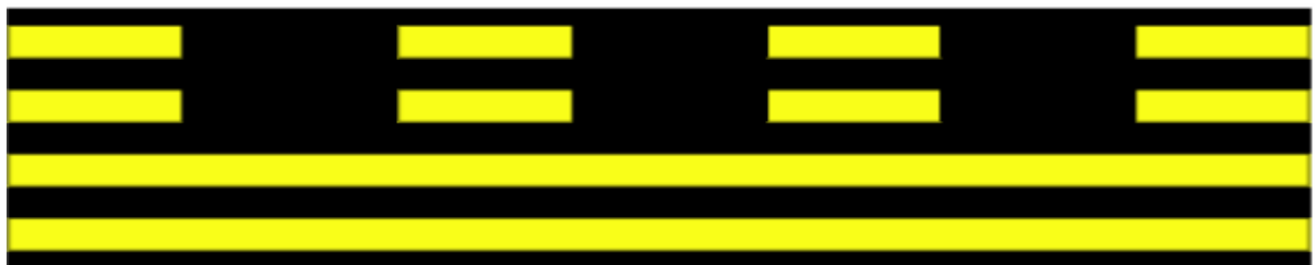
Figure – 4 Runway Holding Positions Markings
