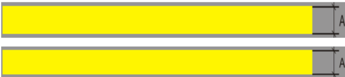
Figure – 2 taxiway edge marking and dimension
