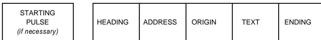
**Figure 4-2. Form of transmission — teletypewriter operation (*see* 4.4.10.1.2)**
